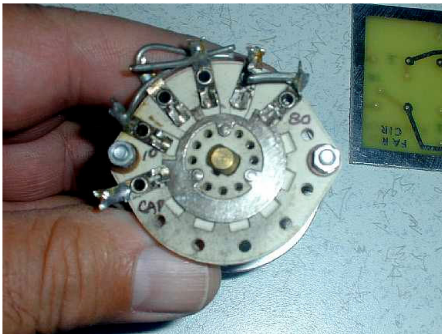
Figure 3: Orientation of bandswitch solder tabs
