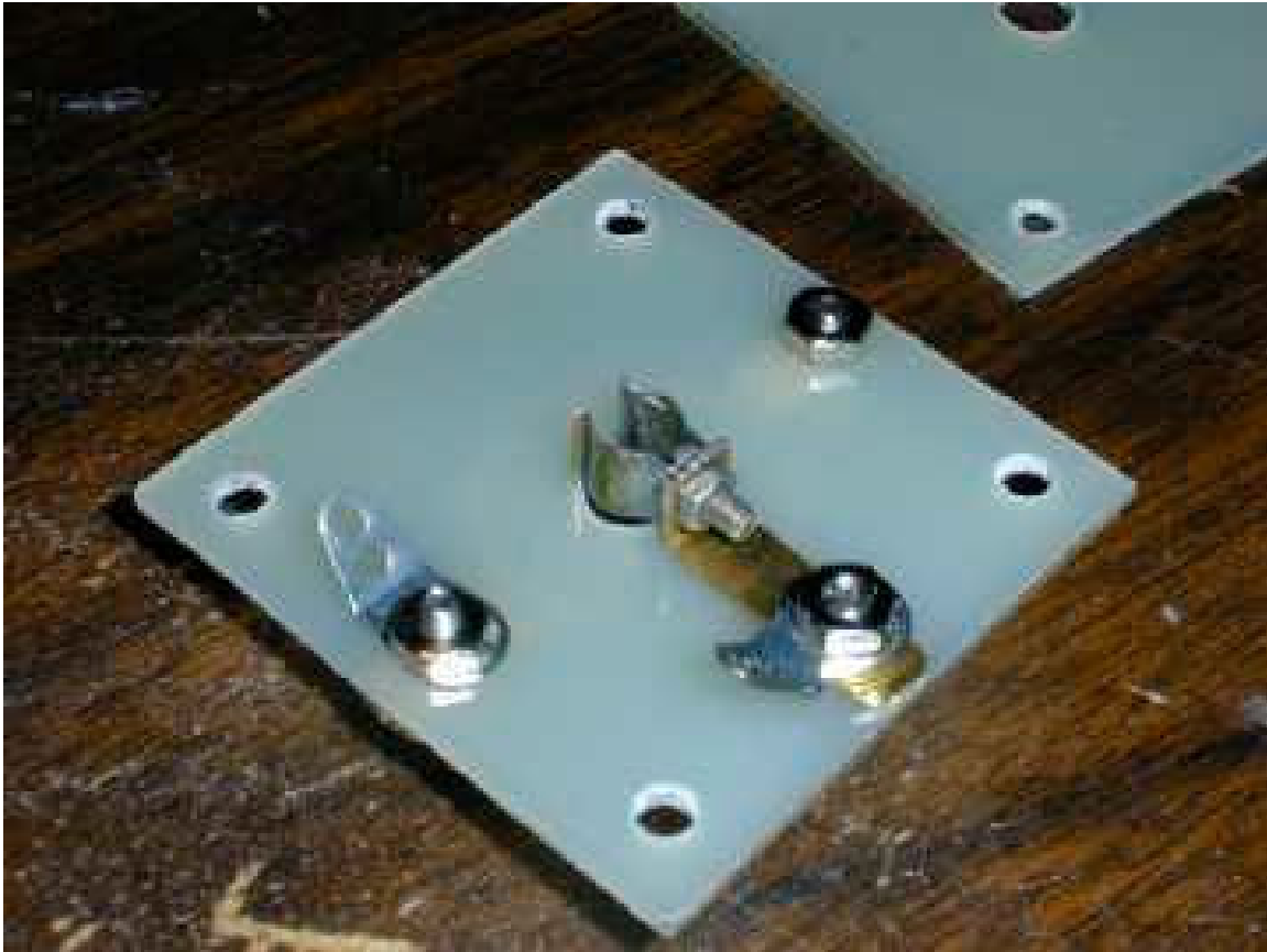
Figure 3: Attaching fuse clip assembly to board
