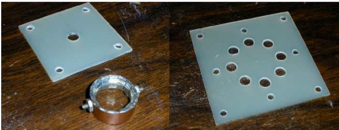
Figure 2: Top and bottom socket blanks with holes 1 3/8" hole not drilled yet
